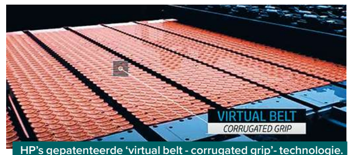
HP's gepatenteerde 'virtual belt - corrugated grip' technologie.
